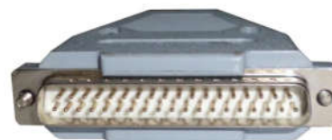
Plug of DB37 ( pin type)
