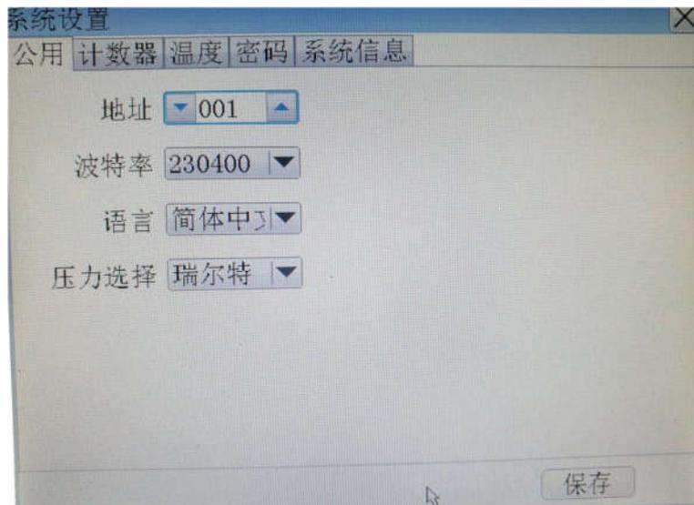
Set the address and baud rate to modify the communication parameters with other controllers such as computers.
