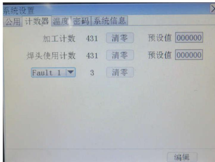
Processing count: the number of welded joints, and the processing count exceeds the preset value, the device will automatically alarm.
