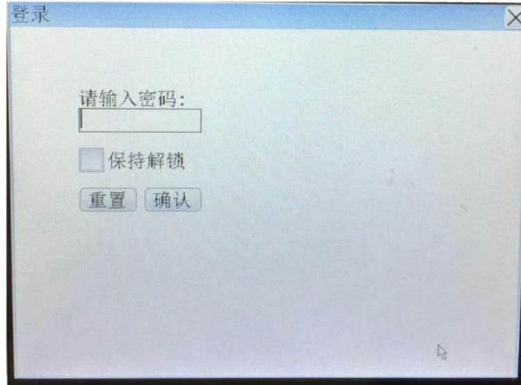
Keep unlocked: After selecting Keep unlocked, you can directly edit without repeating the password, but keep unlocked will be automatically eliminated after power off.
