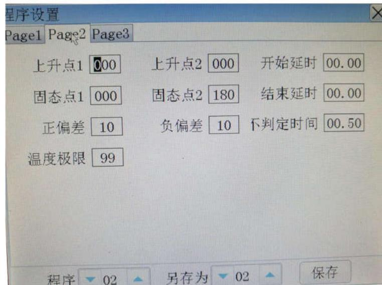
Rising point 1 , 2 : When the temperature rises to this point, a signal will be output.
