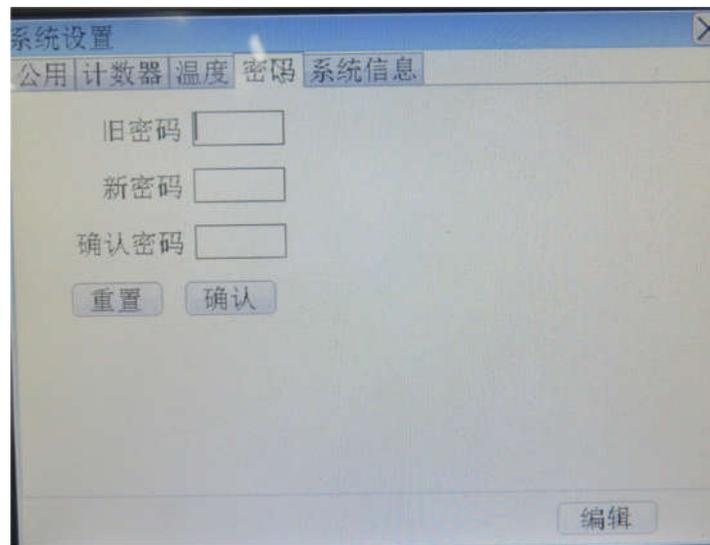
This interface is used to reset the old and new passwords. The original password is: 666666 . Click on the input area and the numeric keypad will automatically pop up to enter the password.
