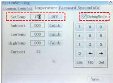
3. Enter the temperature count value as shown in the figure below.
