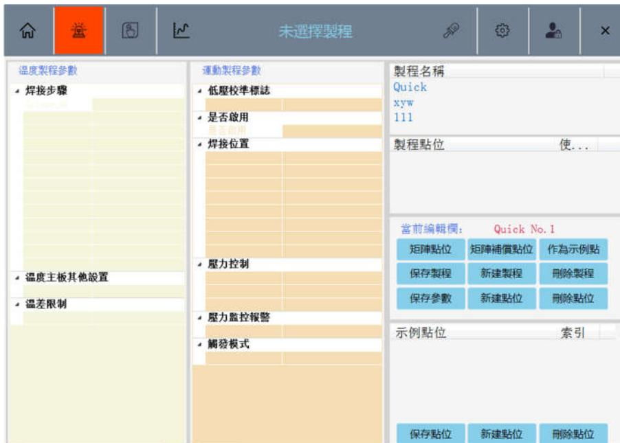
New process steps: 1) Click "New Process" and a dialog box for inputting process name will pop up, and users can input the name according to their needs.
