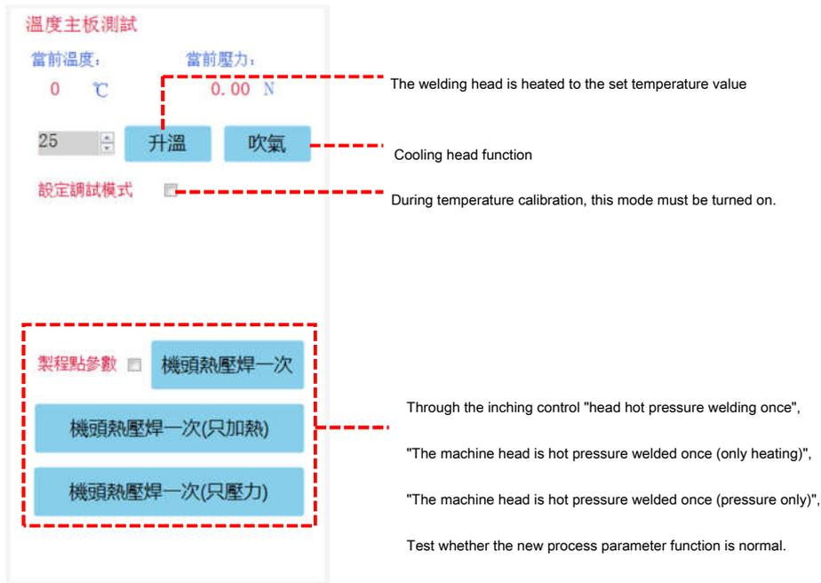
When creating a new process and equipment debugging, this interface is used to test the abnormality of the corresponding function of the temperature motherboard
