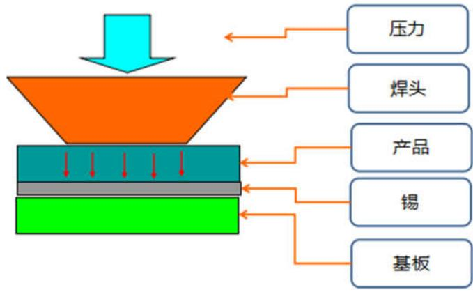
Pressure control adopts dynamic closed-loop control mode, as shown in the figure below.
