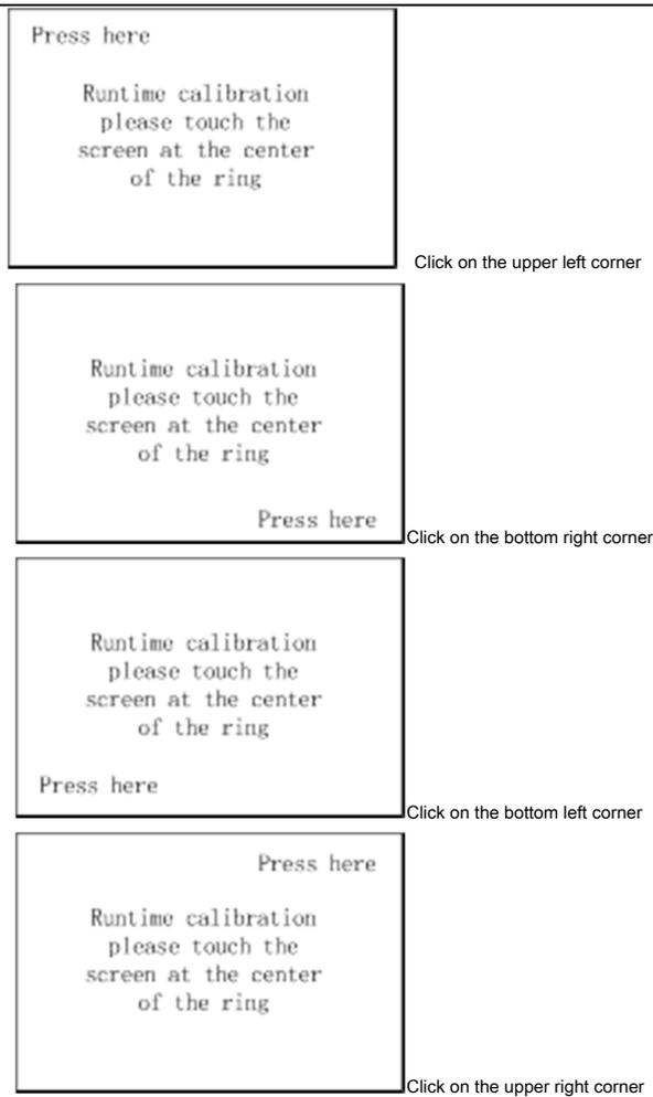
After completing the above four-point calibration, click the middle point of the screen to automatically complete the touch screen calibration.
