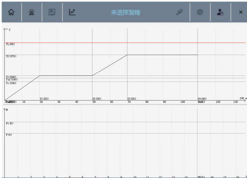
Real-time display of temperature and pressure curves.
