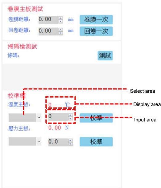
The roll film main board test can be divided into three parts: roll film main board test area, scan code gun test area, and calibration bar.
