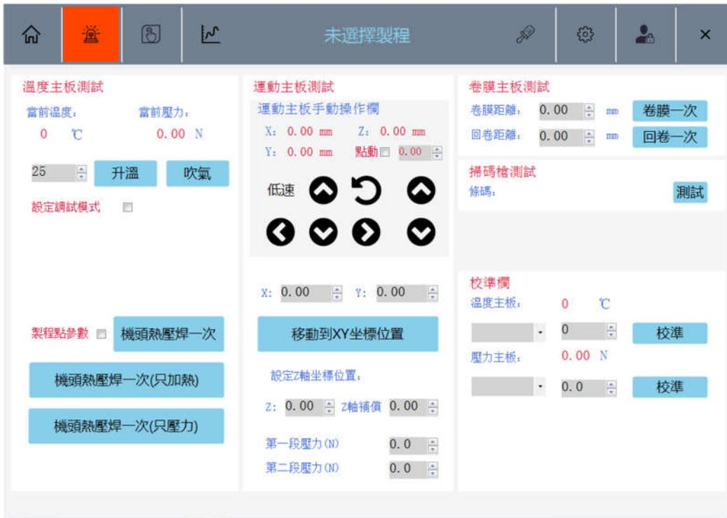
The manual interface can be divided into three parts: temperature mainboard test area, sports mainboard test area and roll film mainboard test area.
