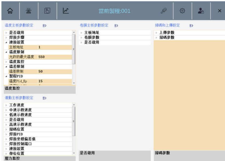
The setting interface can be divided into four parts according to function: temperature motherboard parameter setting, sports motherboard parameter setting, roll film motherboard parameter setting, and so on.
