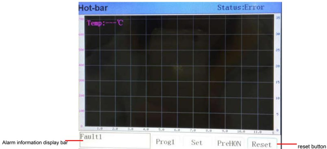
Remarks: After the alarm information is eliminated, click the "Reset" button to confirm the alarm!
