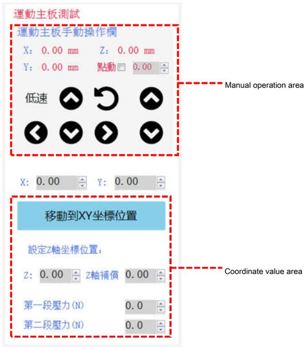
The user can test whether the function of the motion board is normal by moving the motion axis. There are two ways to move the motion axis: 1) Jog through the manual operation area
