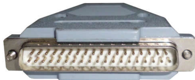
Plug of DB37 ( pin type)
