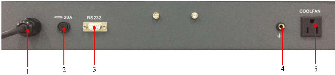
1. Power inlet module: connect 220V AC (refer to nameplate) power into power inlet module.
