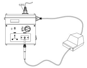
(4) Measure the resistance between the soldering iron tip and ground
