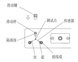
1. Press the sliding key in the direction indicated by the arrow and install the sensor (red-ended connection marker
