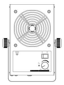
The series BLOWER PC ionized air blower produces an air flow that is rich in positive and negative ions. Directing the air flow on an object that has a static electricity charge will neutralize the charge. If the object has a negative static charge, it will draw positive ions from the air flow. Conversely, if the object has a positive static charge, it will draw negative ions from the air flow. The air ions are attracted to the oppositely charged object and neutralize the charge on the object.
