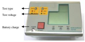
Test type LED: green is surface resistance test, unit: ohm/m²
