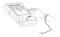
(1) Wear a good WRIST band, the WRIST band cable directly into the WRIST with jack (WRIST CORD) or connected to a connection column.
