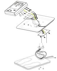
Fixed columns: after connected at the bottom of the well, remove the package of three 6 x 25 hex socket screws, according to the icon will be fixed on the column base plate, the post tighten screw.
